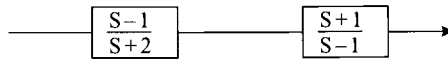
Figure 7.19 An obvious strategy to cancel an unstable pole by a zero at the same location in the s plane
