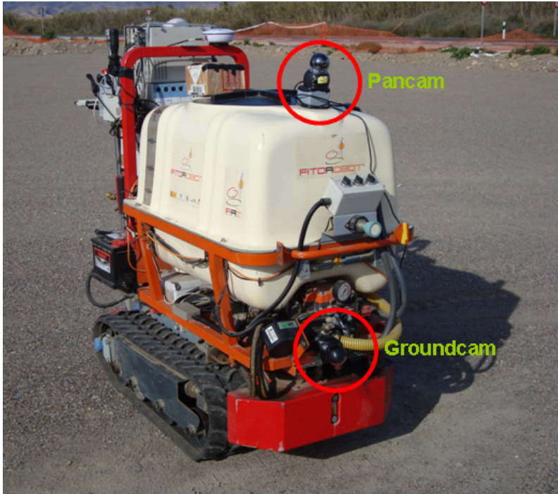
Fig. 3.6 Tracked mobile robot Fitorobot during physical experiments (notice the cameras Quickcam Sphere AF, Logitech)
