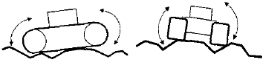
Fig. 1.4 Tracked locomotion on bumpy (or 3D) terrains [47]
