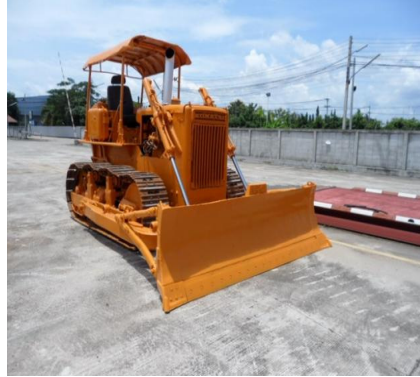
(b) Komatsu bulldozer D50, applied to construction and mining (year 1947) [97]
